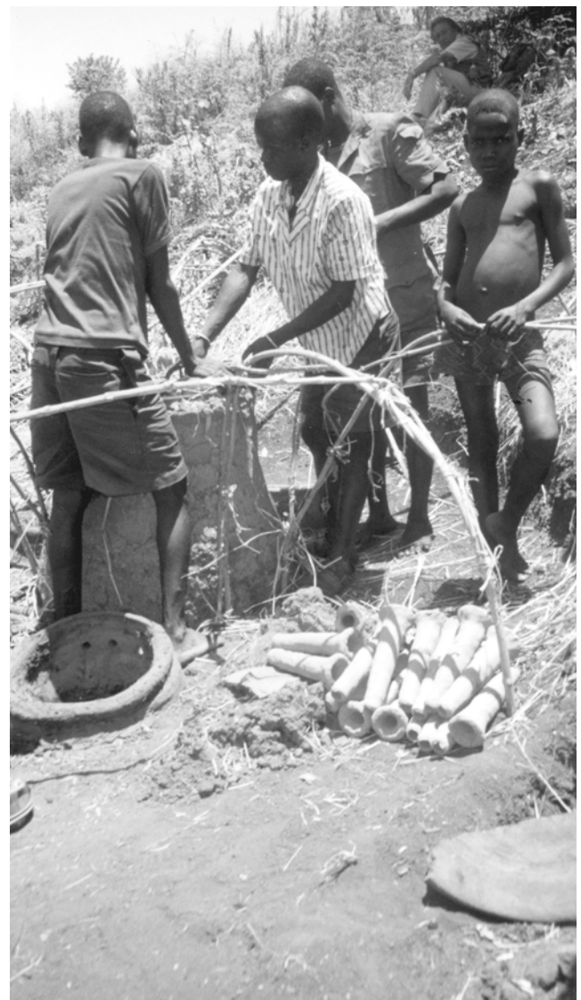
Figure 2. The furnace and pot bellows are repaired and ready for smelting (photo. Gunnar Haaland).
