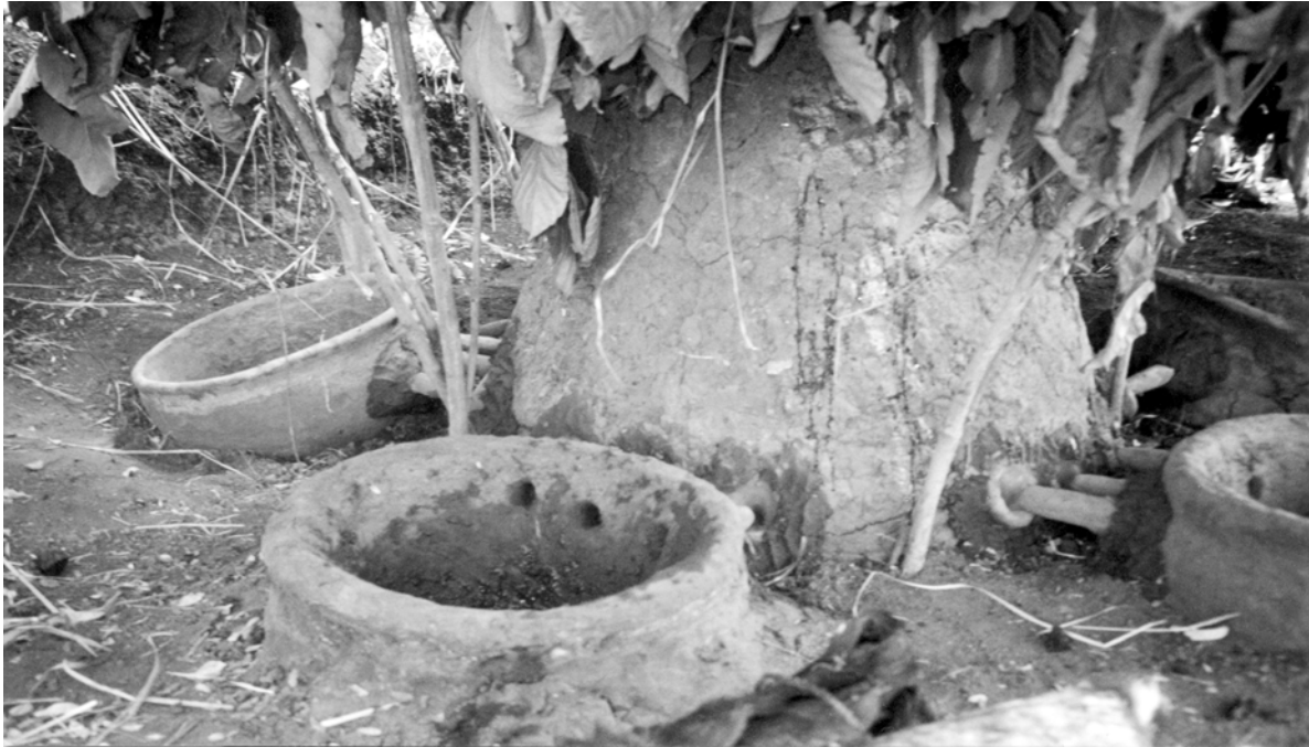
Figure 4. The two types of tuyeres are attached to the pot-bellows and furnace (photo. Randi Haaland)
